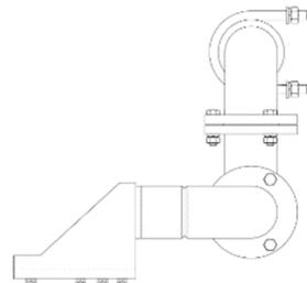
Front cleaning device under Cab
