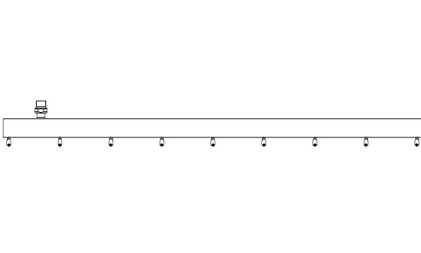
Low-pressure front cleaning device under Cab
