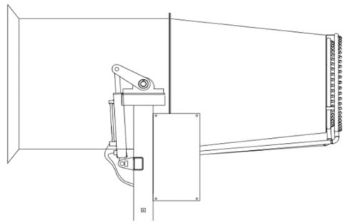
Air Supply Type Sprayer on rear work platform
